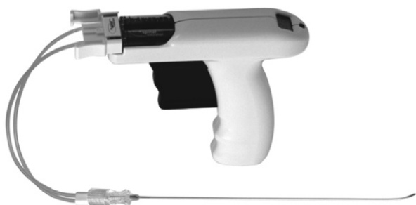
Figure 1 The Biostat Delivery Device is a hand-held delivery system that separates the reactive thrombin and fibrinogen solutions until just prior to delivery into the target disc. A digital pressure manometer allows the user to monitor intradiscal pressure during fluid delivery. When mixed, the liquid components can flow through the disc and anular fissures before rapidly transforming into a dense gel-like, three-dimensional microporous fibrotic matrix of fibrin.
